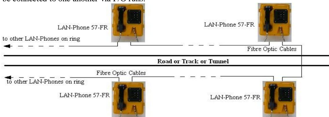
A more detailed section of a typical F/O Ring can be seen in the diagram above.
