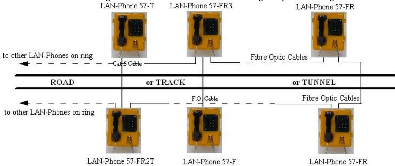
57-FR2T variant of the telephone to have an additional telephone "T" connected to it via Cat 5 cable. This can be a very useful facility especially where existing cable ducts are in place. An alternative is to use the 57-FR3 variant of the telephone when it is possible to have an additional F/O telephone "T" connected to it via a F/O cable.
