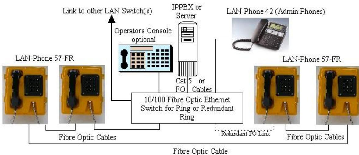
Redundant ring structures can be built up using the F/O ports of the LAN-PHONE 57. The figure above shows a redundant ring structure with LAN-PHONE 57 equipment. To construct a ring the first piece of equipment is connected to the last in the fiber optical line structure consisting of LAN-PHONE 57 equipment and the redundant fiber optical ring closed. Note: All the telephones in the redundant ring may only be connected to one another via F/O runs.
